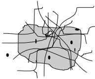
Figure 10.1. Effect of the filamentous organisms on the structure of the activated sludge floc (EPA, 1987)
